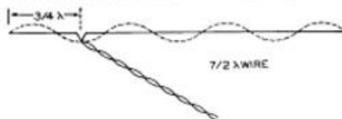
Figure 22 Method of Feeding a Harmonic Antenna with a Twisted Pair When It Is Physically Impossible to Center Feed It.
