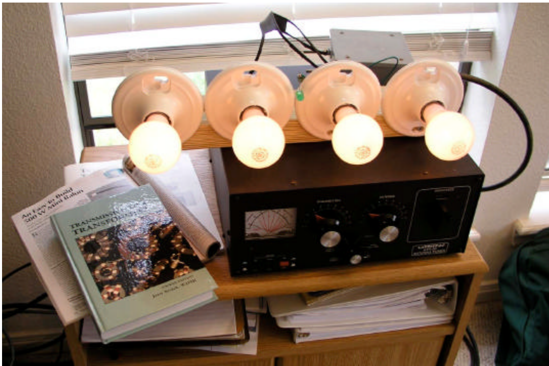
4 X 100 W Bulbs for a 200 Ohm RF Load
