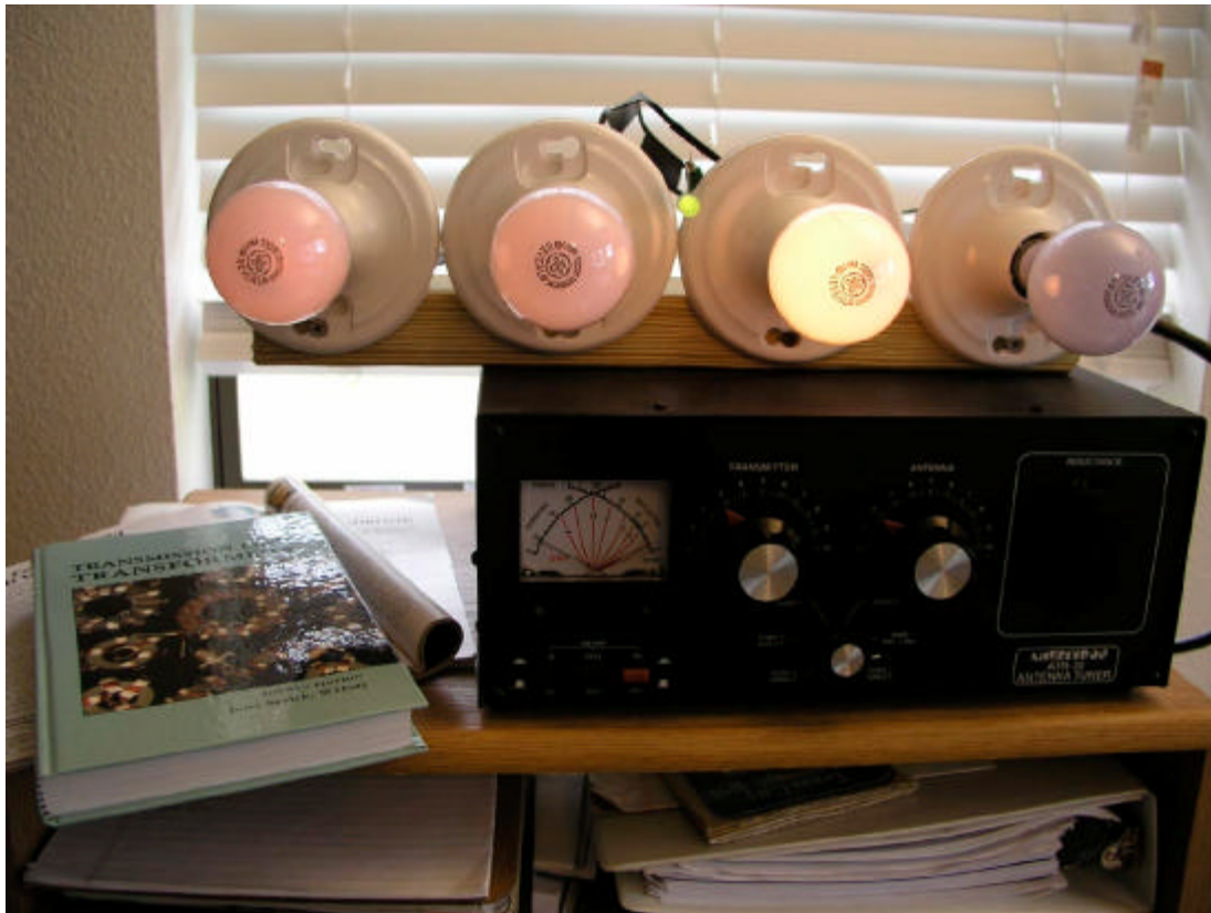
The Green LED Shows Unbalanced Load Condition with one bulb shorted
